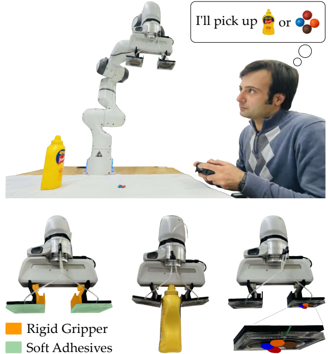
Fig. 1. Human controlling an assistive robot arm and RIgid-SOft (RISO) gripper. The RISO gripper is formed by mounting soft, switchable adhesives to the bottom of a rigid, industry-standard, parallel mechanism. Using RISO grippers robot arms can pick up large, rigid items (e.g., a jar of mustard) as well as small, numerous, and fragile objects (e.g., a pile of candy).
